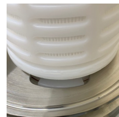
Lugs incorrectly positioned
